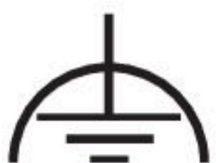
FIGURE A.4.5.2(b) Symbol that Represents Functional Earthing — IEC Symbol Number 5018.
