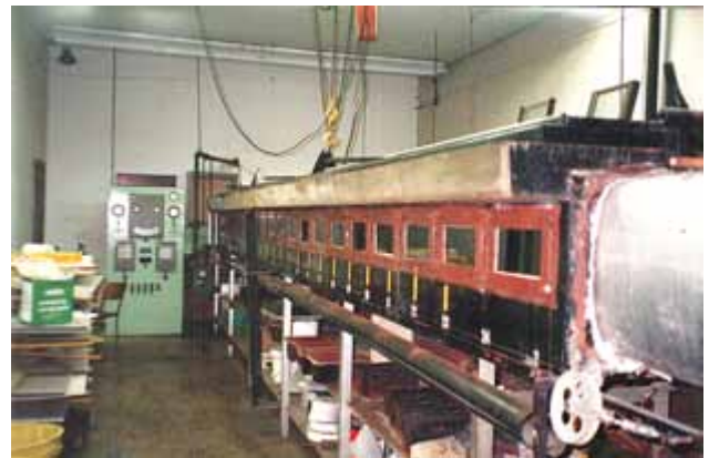
ASTM E84 room tunnel test apparatus. (Photo courtesy of Herbert Blenstein)
