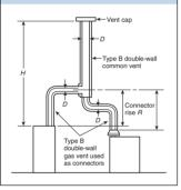
See Annex F for diagrams and more information on how H and other dimensions called for in the venting tables are measured.
