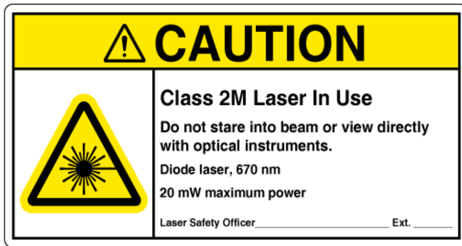
Figure 1b. Sample ANSI Z535.2 & ISO 3864-2 Compliant Class 2, Class 2M or Class 3R Laser Controlled Area Warning Sign
