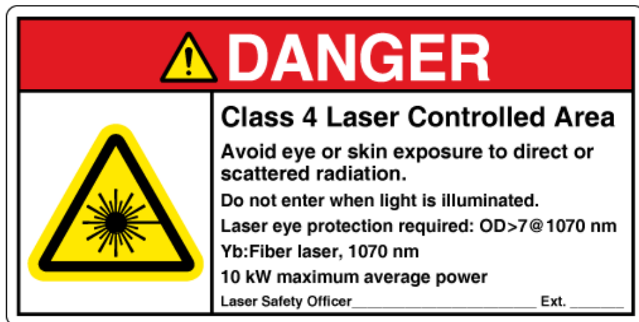
Figure 1d. Sample ANSI Z535.2 & ISO 3864-2 Compliant Class 4 Laser Controlled Area Warning Sign
