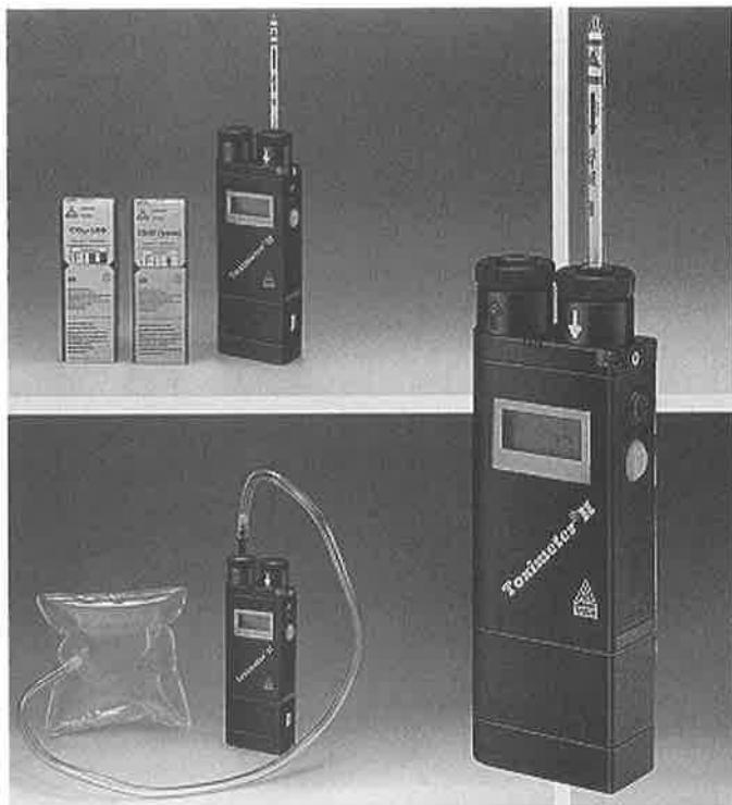
INSTRUMENT 17-30. MSA Kwik-Draw Deluxe and Toximeter II Detector Tube Pumps.
