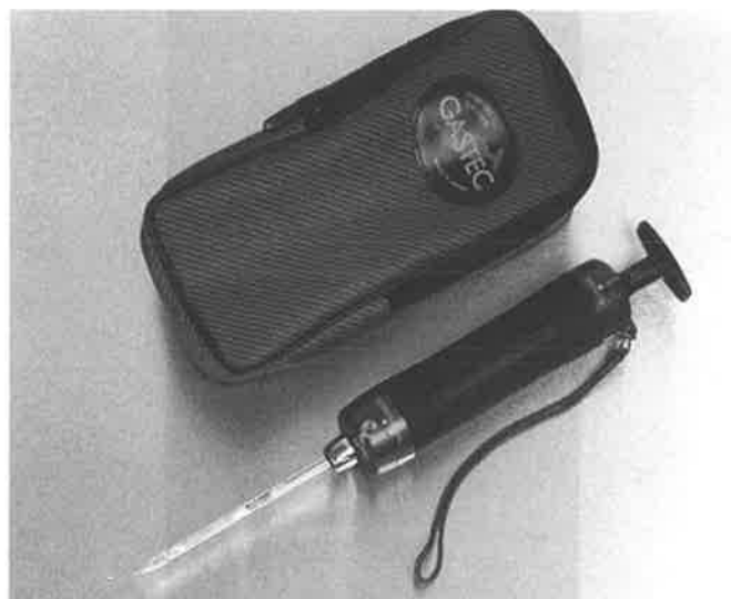
INSTRUMENT 17-37. Sensidyne/Kitagawa Qualitative Multistage Tubes.
