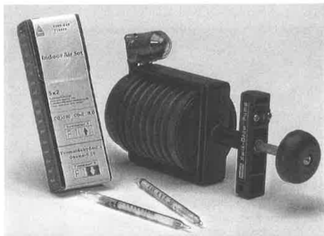
INSTRUMENT 17-32. MSA Indoor Air Quality Kit.
