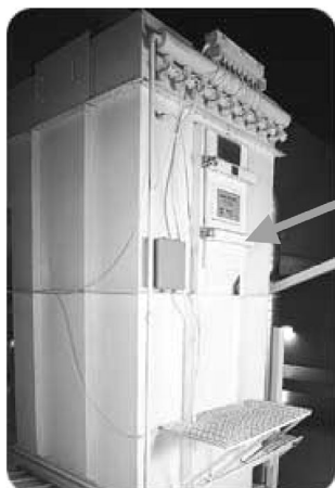
FIGURE 6-7. Side access, bottom bag removal design
